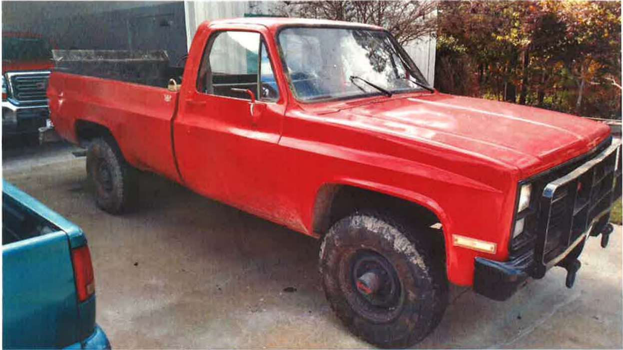
Photo shows the bent brush guard believed to be impacted by the DOT sign also you can see the missing windshield wiper blades and right side mirror is missing.
